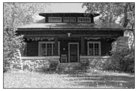
The full-width, open verandah with fieldstone on the lower part of the wall and a roof supported by fieldhouse pillars and logs.
