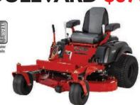
Engine 23 hp Kohler® KT730 Hydro-Gear® ZT-2800 Drive System Fuel Capacity 5 Gallon Joystick or Twin Lever\* Steering Control 20x10-10, 20x12-10 Tires. Rear 13x6.5-6 Tires, Front Ground Speed 7.5 mph Front Axle Fixed Cutting Width
