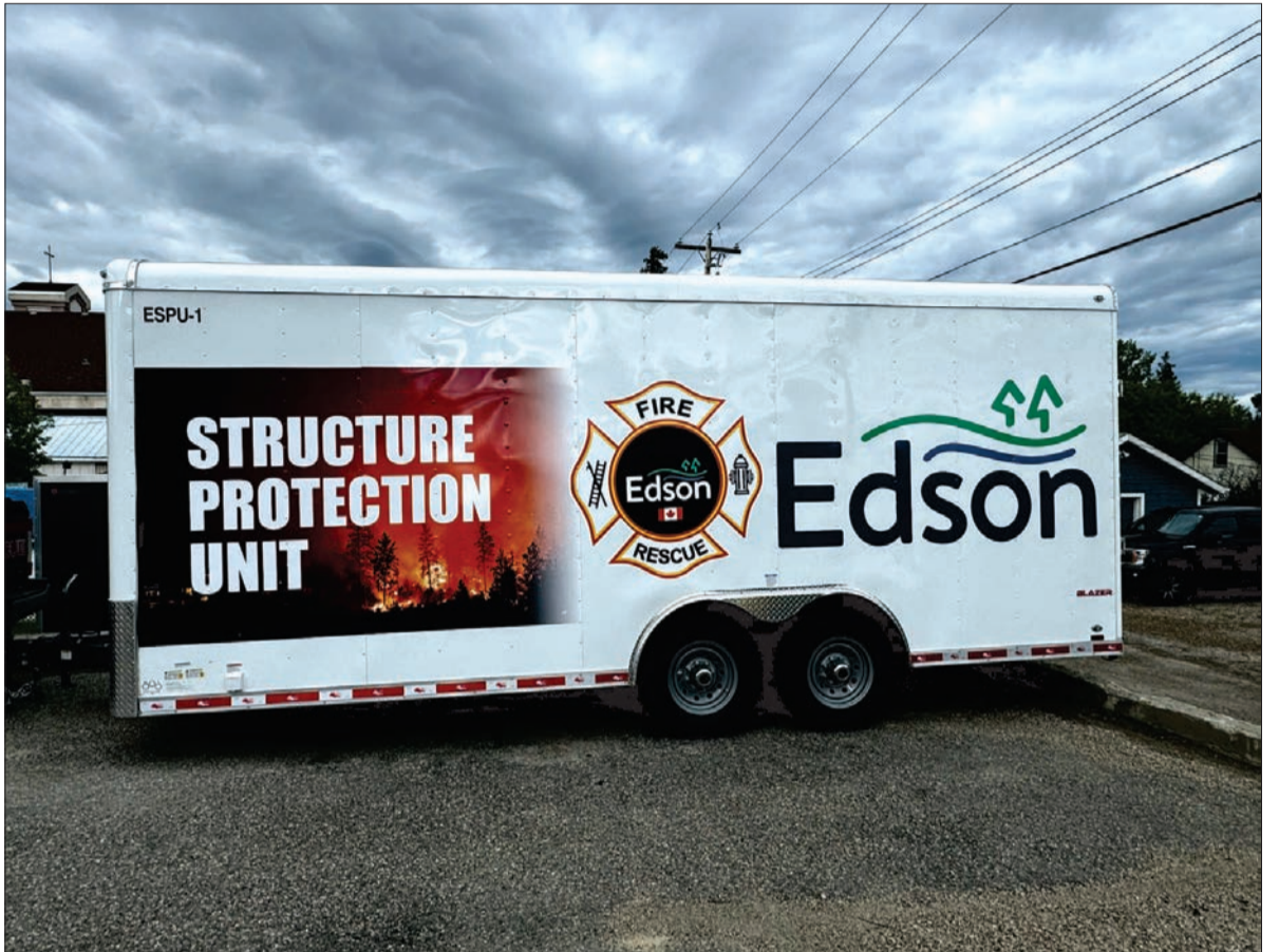
The Town of Edson's new Structural Protection Unit consists of pumps, sprinklers, hoses, and other equipment that can be quickly deployed to protect buildings and structures in the event of a spreading fire.
