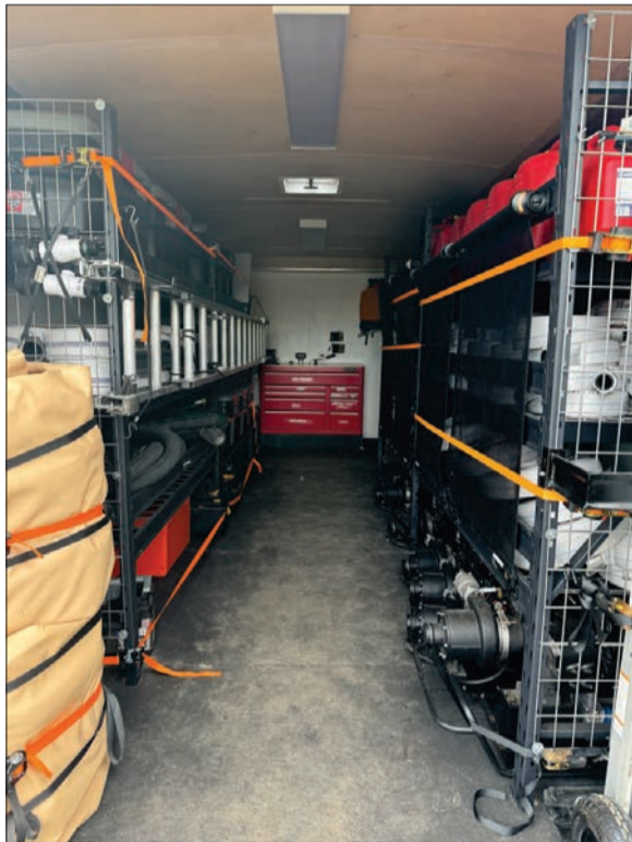
The Town of Edson's new Structural Protection Unit consists of pumps, sprinklers, hoses, and other equipment that can be quickly deployed to protect buildings and structures in the event of a spreading fire.
